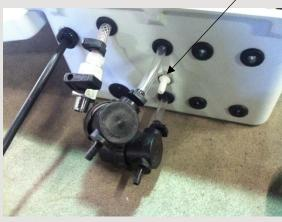
First, screw your Y-connectors (HY14AS QTY: 2) into the ends of the foam chambers with a wrench.
