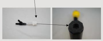
Then connect your 1/4" tubing lines (VL0140) to each "Y" connector (both ends as pictured), and run the lines along the boom frames toward the tank/compressor assembly. Cut the tubing accordingly for each line. Make sure there is excess tubing where your spray boom folds up to prevent the lines from getting tangled.
