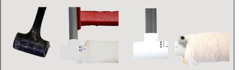
Hammer the sponge white caps into the t-risers until the edge of the white cap reaches the center of the t-riser. Remove the red cap after hammering and shine a flashlight through the riser to make sure your cap has reached the center of the t-riser as shown below.
