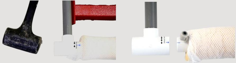
Hammer the sponge white caps into the t-risers **until the edge of the white cap reaches the center of the t-riser**. Remove the red cap after hammering and shine a flashlight through the riser to make sure your cap has reached the center of the t-riser as shown below.
